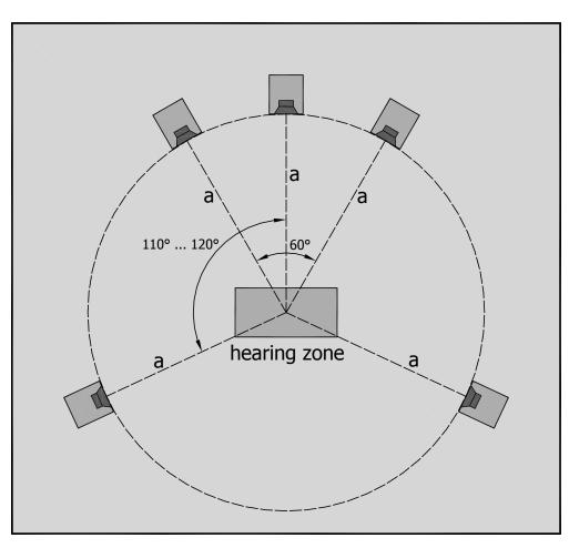
• Distance between speakers and your listening position  $a = 2.5 \text{ m} \dots 5 \text{ m} (8'2'' \dots 16'5'')$ In case installation in the prescribed way is not possible in your listening room most decoding devices allow adjustments of single speakers.
